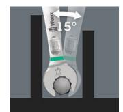
The Joker 6005 double open end wrench with its special open end design - a 7.5° offset open end and double hexagon geometry - doubles the placement points at a repeated 180° rotation of the wrench around the longitudinal axis. Bolts and screw heads can be engaged every 15°. The Joker 6005 will automatically find the respective placement point after every turn.
